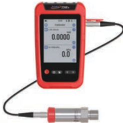
Additel 226Ex with ADT161Ex Pressure Module
